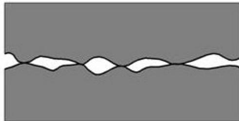
Figure 1 - Contact occurs only at A-Spots, regardless of the overall interface geometry.
