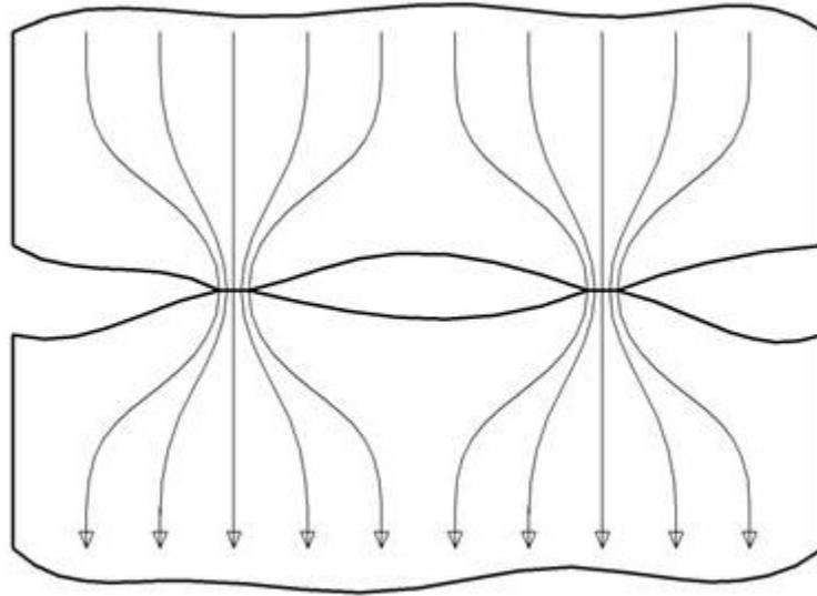
Figure 5 - Current flow constricts in multiple parallel pathways through the A-Spots.
