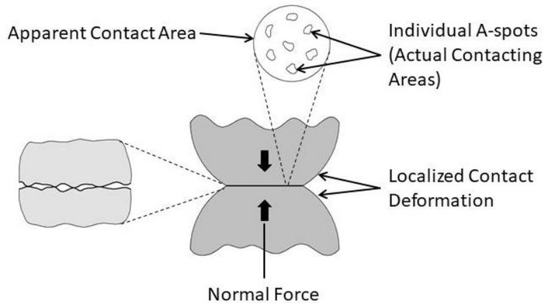
Figure 3 – A-spots distributed within apparent contact area, provided by overall interface geometry.
