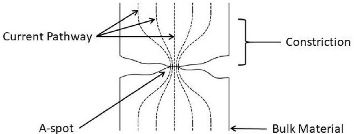
Figure 4 – Current follows a constricted path from the bulk material to an interface A-spot.
